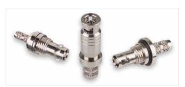
The new Mini HD-BNC plug requires much less space than its predecessor. It saves more than 40 % of space. For applications in plug panels and patch panels on which many connections are used in matrix form within a limited space, it allows four times the packing density in comparison to the standard BNC. The dimensions and weight of the devices can therefore be reduced considerably.
